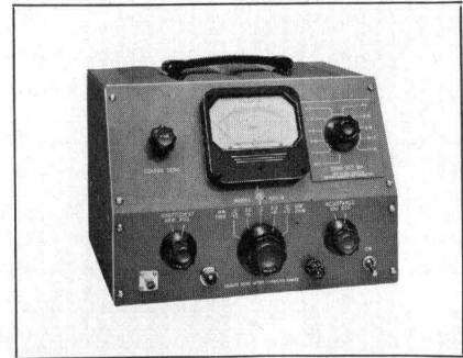
Fig. 7. -hp- Model 430B power meter as modified for use with Model 477A coaxial thermistor mount. New bias current switch is at upper right of panel.
